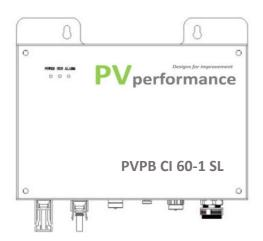
PV Power Booster: As soon as the String Voltage drops down below the adjusted switch-ON Threshold value, the PV Power Booster will set the entire Modules/PV-System on a high Positive Potential against ground. The accumulated PID/HVS degradation during operation of the PV modules will be recovered in this way.
