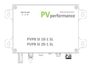
PV Power Booster: As soon as the String Voltage drops down below the adjusted switch-ON Threshold value, the PV Power Booster will set the entire Modules/PV-System on a high Positive Potential against ground. The achieved PID/HVS degradation during operation of the Modules/PV-System will be recovered.
